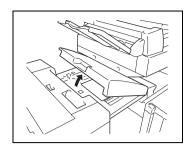
3 Remove any paper, and then close the cover of the horizontal transport unit.
